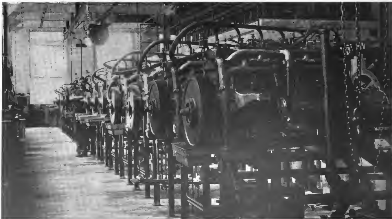
Stevens-Duryea Testing Room—Six-Cylinder Engines in Foreground, Fours in Rear—Electrical Gauges and Testing Apparatus Overhead.
